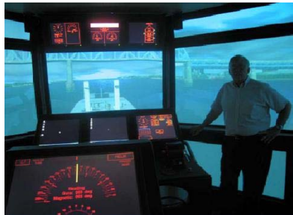
Figure 17 Bridge Mockup and Projected Visual Image
