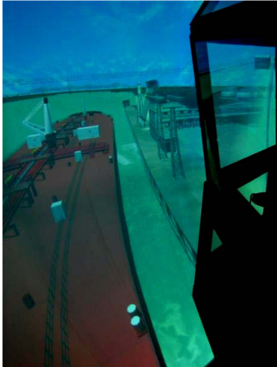
Fig 19 View from simulator entrance walkway showing image wrapping under wheelhouse window. Note image curve due to off-center parallax. Image is optically correct from conning location.
