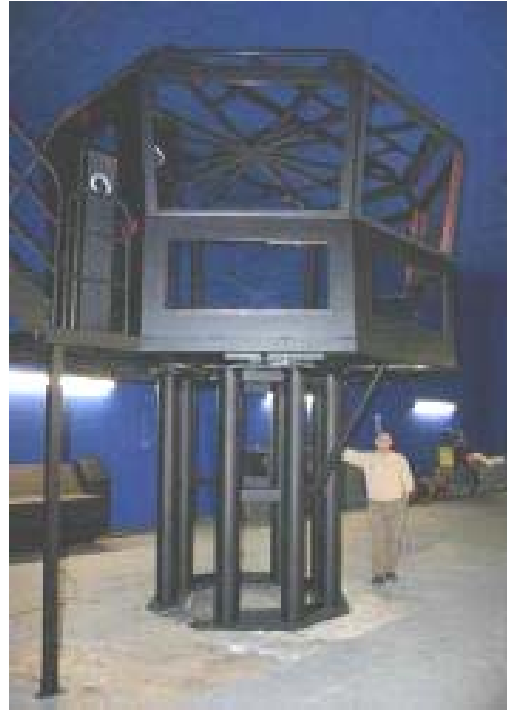
Figure 3 Bridge Mockup Structure Mounted on the Support Posts
