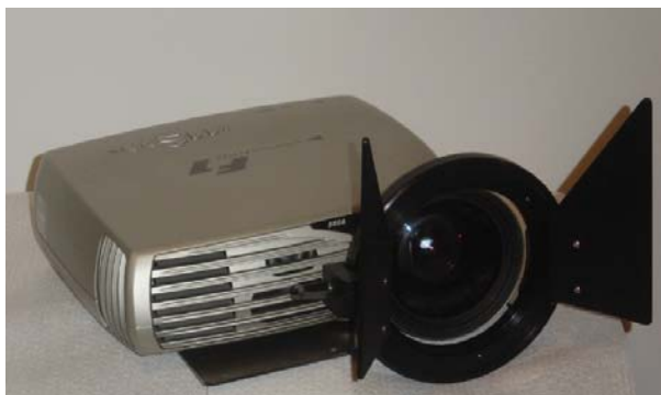
Projection Design SVGA DLP Projector with Wide Angle Lens and Edge-Blend Bat Wing Baffles (Black Level Enhancement filter not shown)
