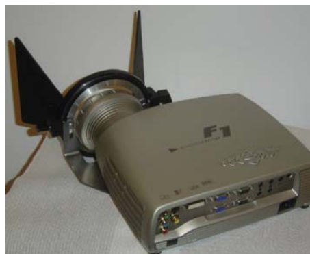
Projection Design SVGA DLP Projector with Wide Angle Lens and Edge-Blend Bat Wing Baffles (Black Level Enhancement filter not shown)
